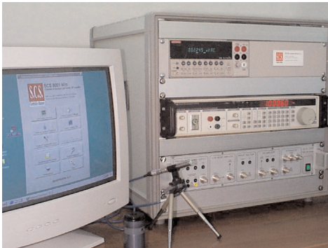
SCS 9001 test bench typical setup
