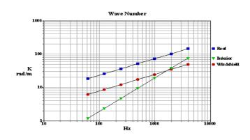
• graph the Wavenumber for the selected subsystems and observe that the glass coincidence frequency is much lower than the roof's. The windshield is an efficient radiator on a large frequency band.
