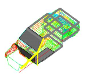
Correlation techniques have to be used with the FEM-BEM methods, between vibrations and sounds, to identify sources and transmission paths while possible noise reduction techniques can be checked out with the possible results.
